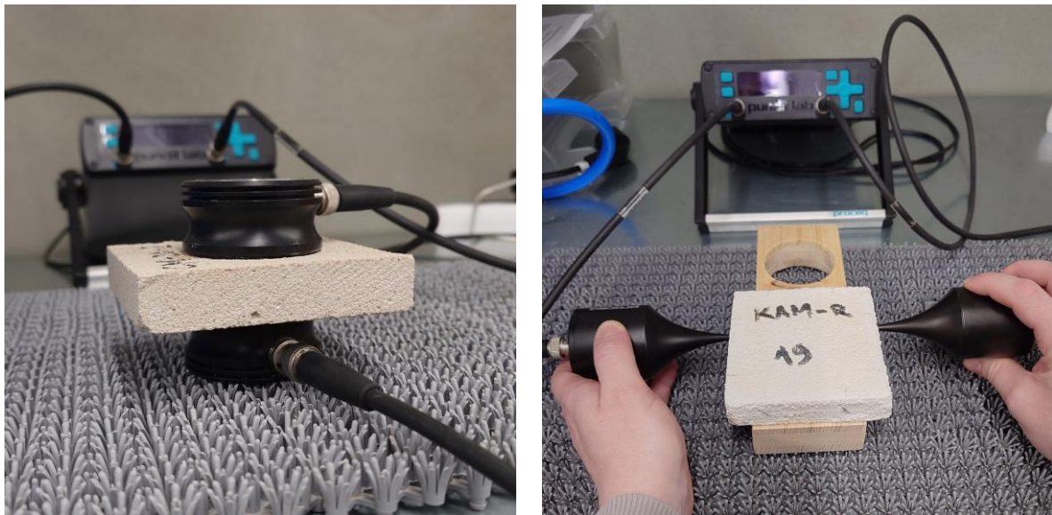
Figure 12: UPV through-thickness test setup (left) and in-plane test setup (right).
