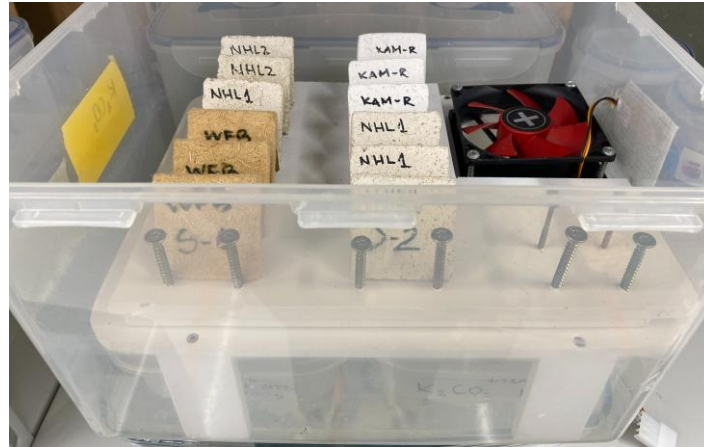
Figure 14: Desiccator used for hygroscopic moisture retention measurements. The specimens were conditioned above a supersaturated salt solution, while an internal fan provided air circulation to promote uniform relative humidity within the chamber.
