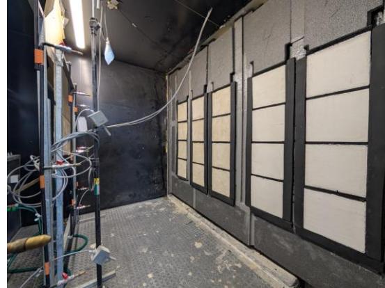
Figure 27. Schematic of the test sample (left) and samples installed in the climate chamber, spray nozzles for rain simulation are also visible (right). (Klöße et al., 2026)
