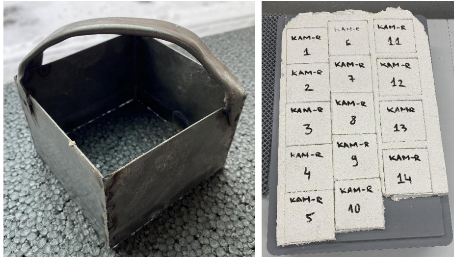
Figure 8: Left: Steel mold used to cut out plaster specimens. Right: KAM-R specimens after drying
