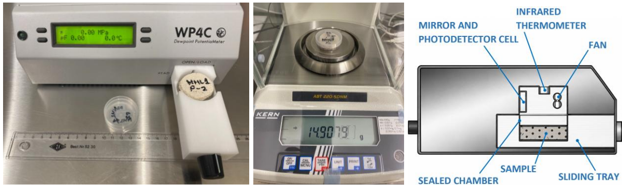
Figure 16: Dew point psychrometer (Meter Group WP4C) used for moisture retention measurements in the overhygroscopic range (left), gravimetric determination of specimen moisture content (middle), and schematic illustration of the dew point psychrometer measurement principle (right).
